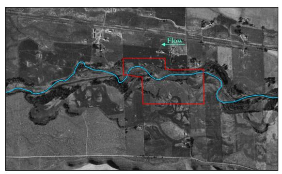
Photograph 23. 1952 Aerial photograph with 1952 river centerline in blue and approximate project area in red. Notice the linear feature downstream of the project area but wide meander belt still present.
